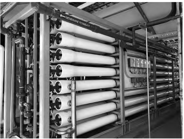
Reverse osmosis membrane units in the Regional Recycled Water Program demonstration facility.
